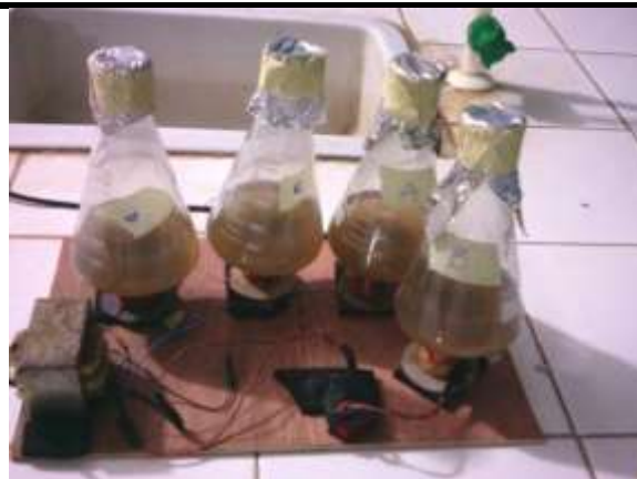
Plate 2: Setup of EMF with wastewater inside the conical flasks during the experiment
